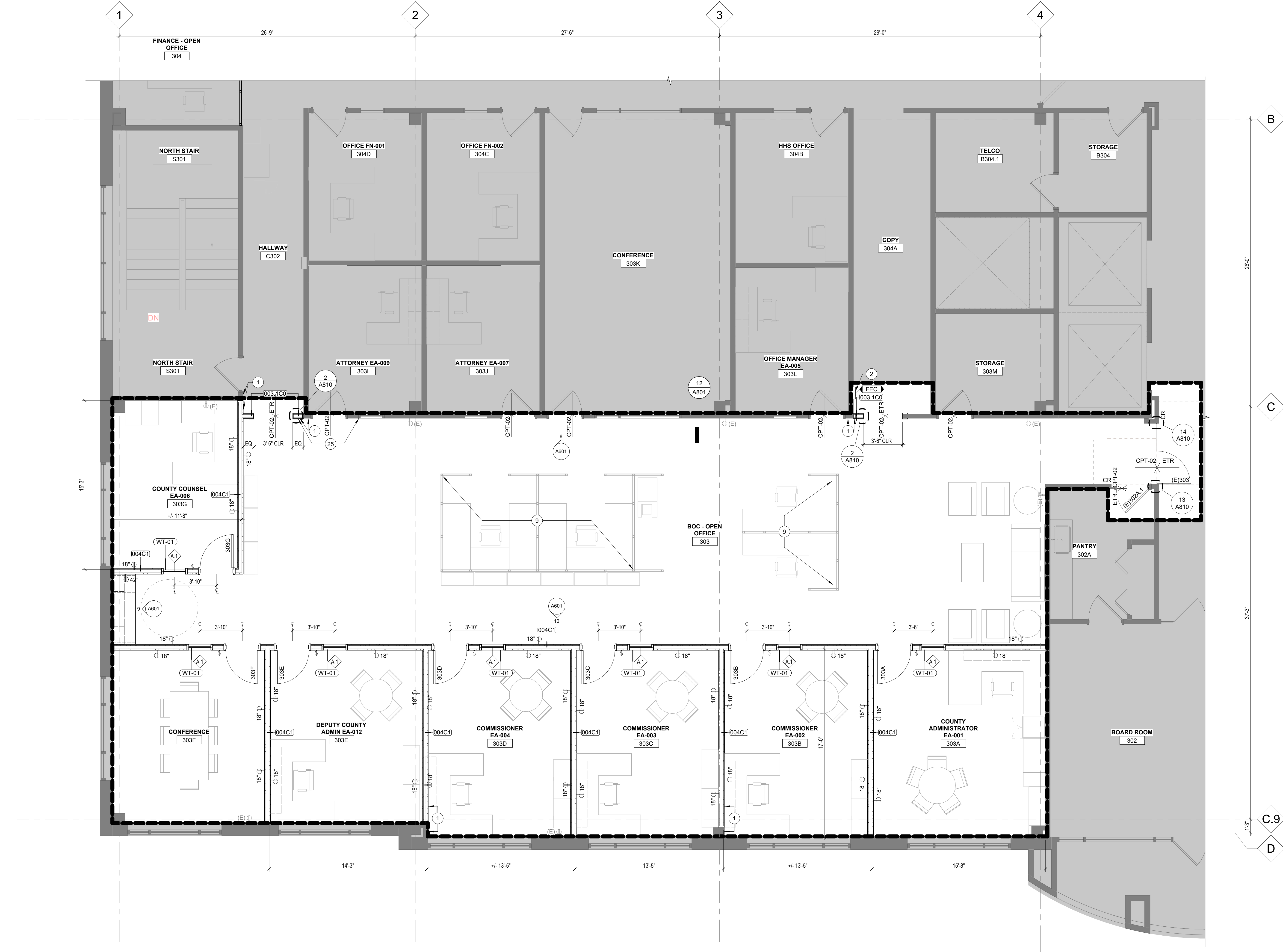
1 ENLARGED PLAN - LEVEL 03 - NW QUADRANT - BOC SUITE 1/4" = 1'-0"
